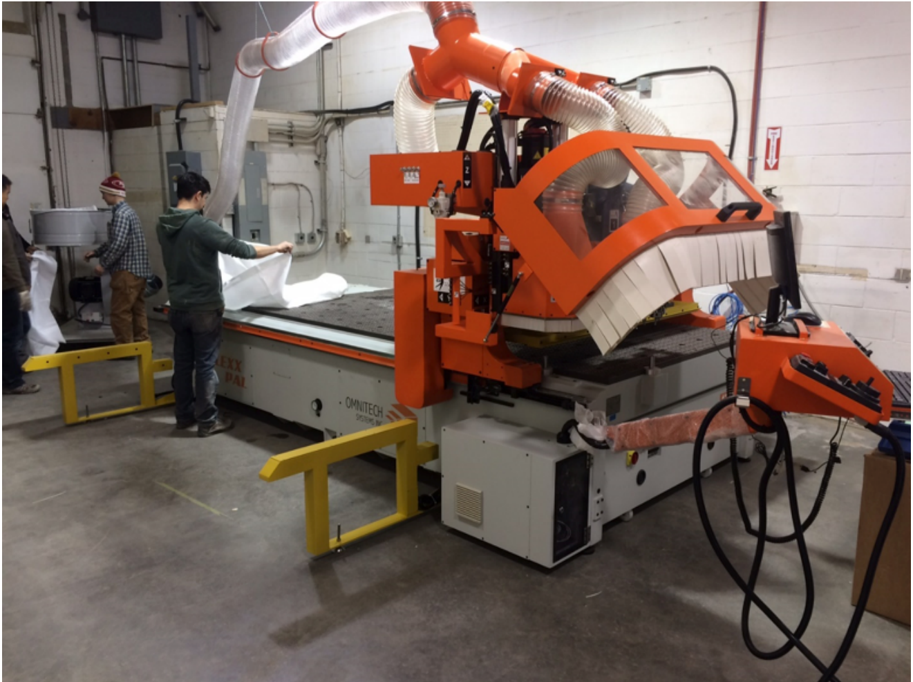
One of Peregrine's CNC machines—a flatbed nesting router.
